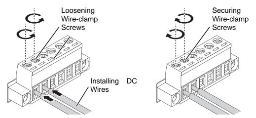
Figure 2.21 Installing DC Wires in a Terminal Block
