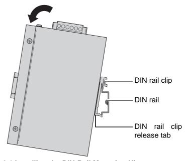
Figure 2.1 Installing the DIN-Rail Mounting Kit
