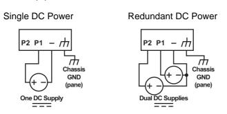
Figure 2.14 Power Wiring for EKI-1242 Series
