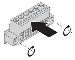
Figure 2.22 Securing a Terminal Block to a Receptor
