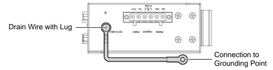
**Figure 2.15 Grounding Connection**
