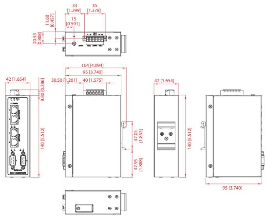
Figure 1.10 Dimensions (EKI-1242BNMS/EKI-1242IBNMS)
