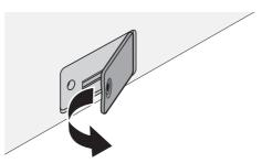
Figure 2.10 Opening the Component Cover
