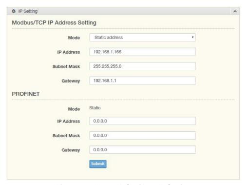
Figure 3.14 Network Setting > IP Setting
