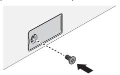
Figure 2.13 Installing the Component Cover Screw
