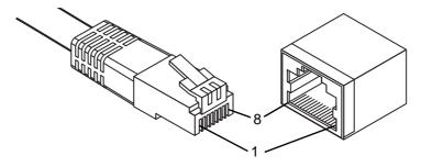
Figure 2.7 Ethernet Plug & Connector Pin Position
