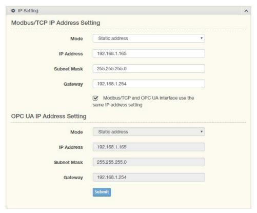
Figure 3.15 Network Setting > IP Setting
