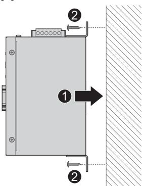
Figure 2.6 Wall Mount Installation
