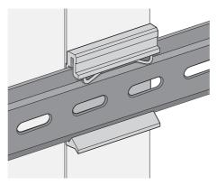
Figure 2.2 Correctly Installed DIN Rail Kit
