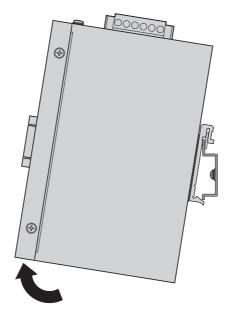
Figure 2.3 Removing the DIN-Rail
