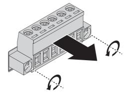
Figure 2.20 Removing a Terminal Block
