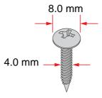
**Figure 2.5 Wall Mounting Screw Dimensions**
