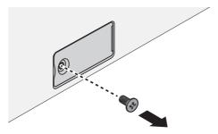
Figure 2.9 Removing the Component Cover Screw
