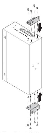
**Figure 2.4 Installing Wall Mount Plates**
