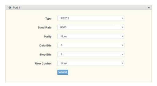
Figure 3.16 Serial Settings > Port 1/Port 2
